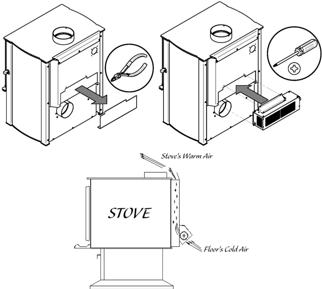
You can also install, on your appliance, a thermodisc #AC05530 (basic model included with the blower), to enable the blower to start or stop automatically when the stove is hot or too cold. It is possible to install the quick connect thermodisc instead #AC02055, sold separately.
