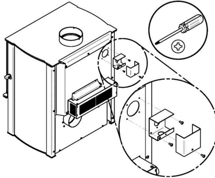
When using the blower without the thermodisc, allow the stove to reach operating temperature (approximately one hour), before turning it on. The increased airflow from the blower cools the firebox and could affect the start-up combustion efficiency if the blower is turned on too early.
