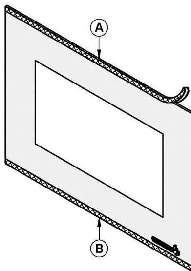
Apply self-adhesive gasket (C) en following the engraving on the inside of the door frame.
