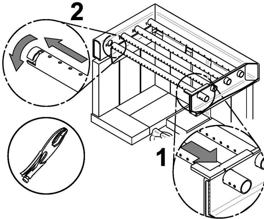
1- Starting with the rear tube, lean and insert the right end of the secondary air tube into the rear right channel hole (**DETAIL 1**). Then lift and insert the left end of the tube into the rear left channel.
