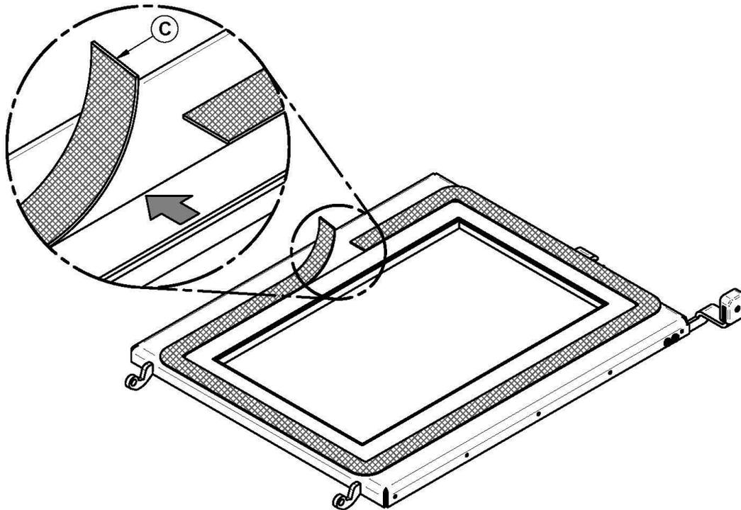
Reinstall the glass, being careful to centre the glass carefully in the door. Do not over-tighten the screws. Note that the two main causes of broken door glass are uneven placement in the door and over-tightening of retaining screws.
